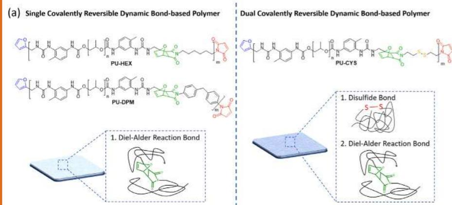
(a) Illustration of the design concept and the chemical structure of PU-DPM, PU-HEX, and PU-CYS.
