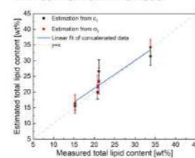
Single microalgae cells were submitted to a rotating electric field to record their electrorotation spectra. Electrorotation spectra were then fitted to the dielectric model with the thickening cell wall to evaluate the cellular composition.
