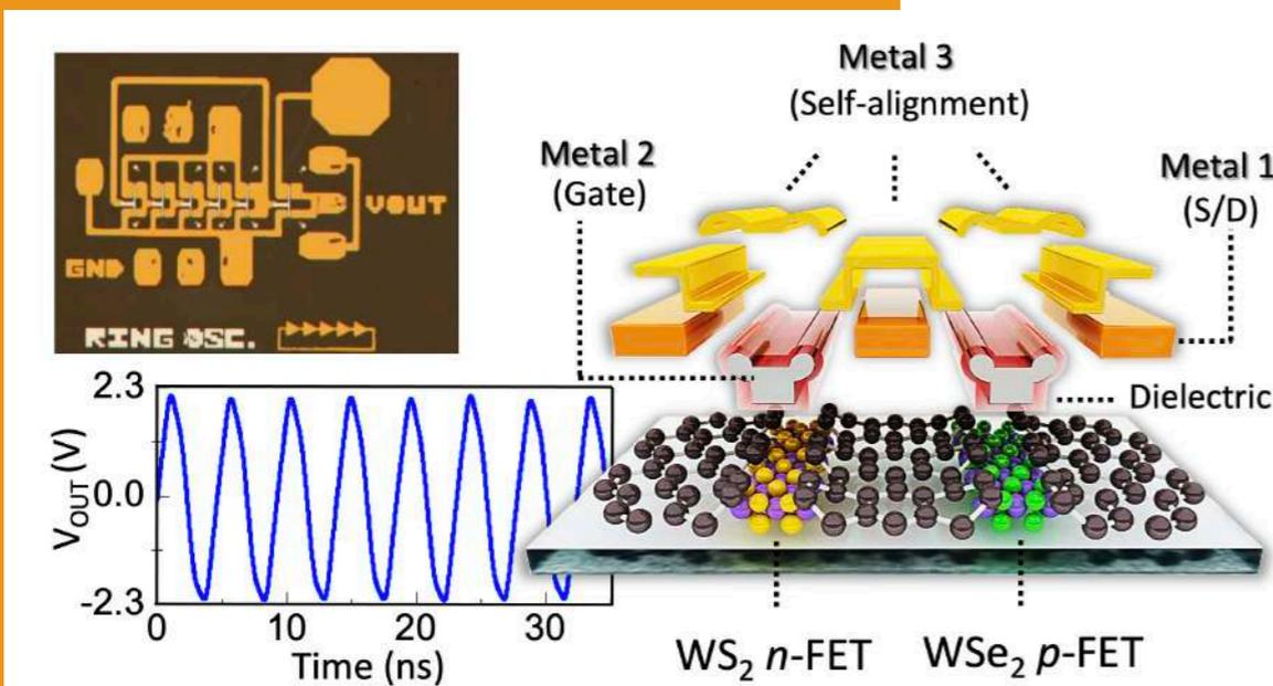
Schematic illustration of 2D FET architecture and measurement property of a ring oscillator thus made
