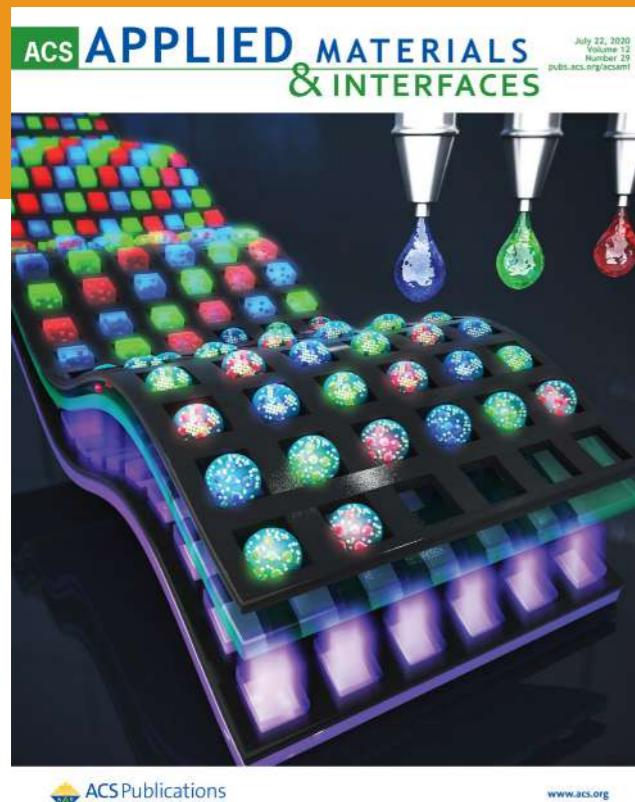
By introducing NaCl into a formulated ink, which enabled spontaneous self-encapsulation of QDs in a single NaCl crystal. An RGB QD@NaCl array with a small pixel size and uniform size distribution (diameter =  $3.74 \pm 0.5 \mu\text{m}$ ) is obtained in the IJP process.
