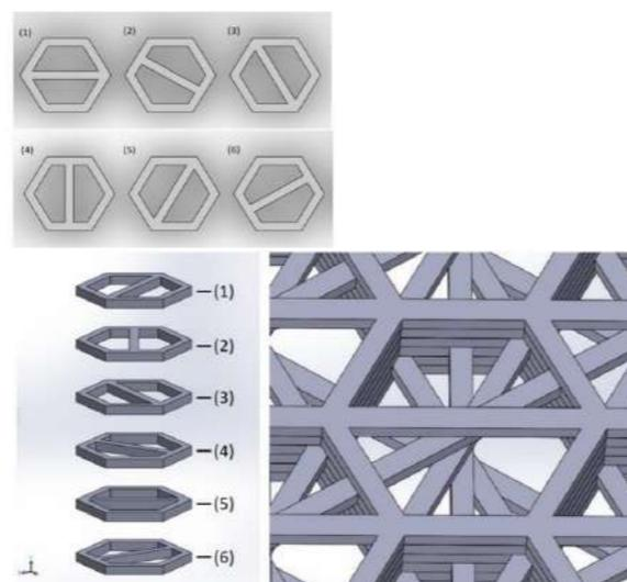
The design and 3D-printed hexagonal stair case scaffolds, seeded with FL83B cells, and cultured for 7 days.
