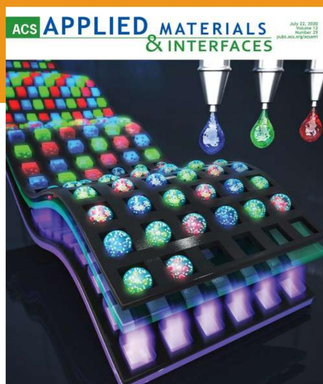
By introducing NaCl into a formulated ink, which enabled spontaneous self-encapsulation of QDs in a single NaCl crystal. An RGB QD@NaCl array with a small pixel size and uniform size distribution (diameter =  $3.74 \pm 0.5 \mu\text{m}$ ) is obtained in the IJP process.
