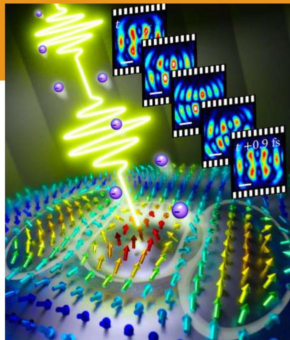
An interferometric photoemission electron microscope is used to time-resolve the vectorial surface plasmon vortex fields and reveal the corresponding spin textures.
